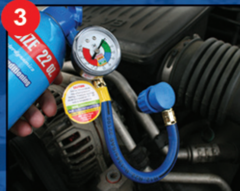
3 Charge AirCon System
