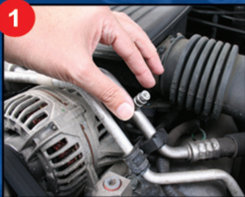
1 Find low-side port and remove cap
