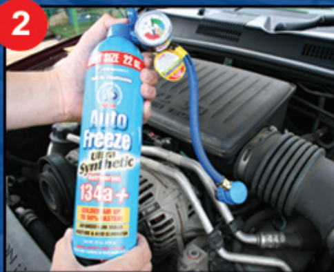
2 Measure AirCon System
