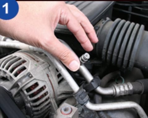
1 Find low-side port and remove cap
