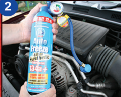
2 Measure AirCon System
