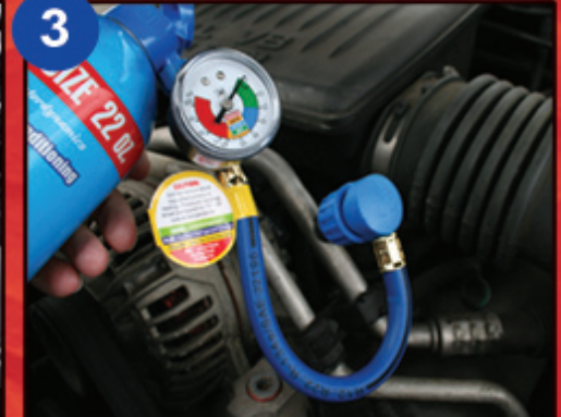
3 Charge AirCon System
