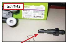
Differences on bleed screw on CSC, also note different colour T.S.B. No.: CL023/09
