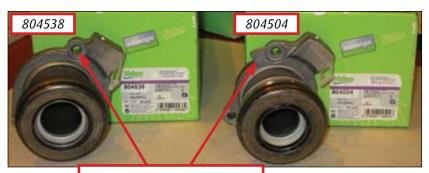
Note the extra casting on 804504 and different location of bolt hole in relation to the hydraulic connector.
