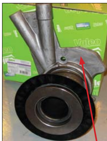
Height sensor removed for manual gearbox
