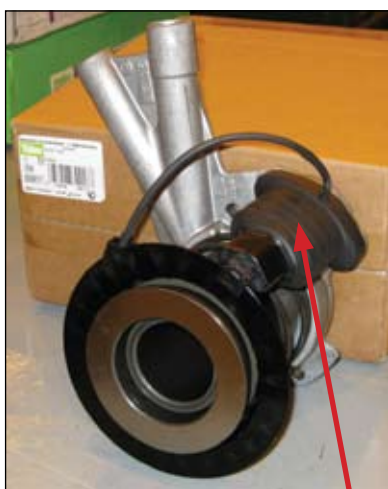
Height sensor for robotised gearbox
