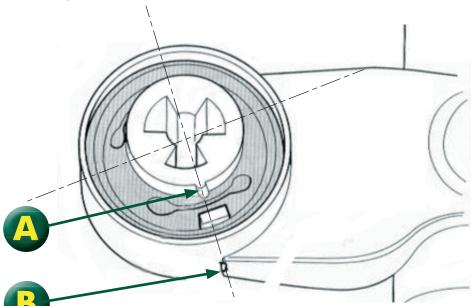
The identifcation mark on the face of the bush (A) must be aligned with the edge of the trailing arm on the axle beam (B)
