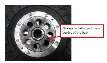
To reduce the chance of this effect, always use the correct, high temperature grease suitable for use in clutch environments. Copper based grease is unsuitable for use due to its low viscosity.
