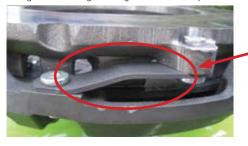
A severe distortion or bend in the drive strap will result in complete loss of pressure plate lift in this area of the cover. This can cause severe gear selection problems.
